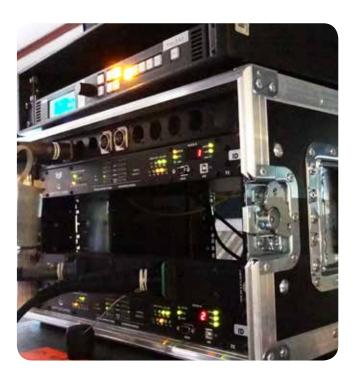
GB4D purchased 4-core fibre cables for the show, which allowed the BroaMan and OPTOCORE rings to share the same cable infrastructure; although the two systems worked independently, the cabling cost was massively reduced.
