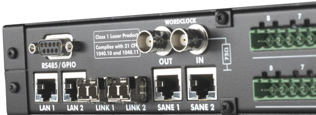
Image:- X6R-FX 'bridging' device featuring both OPTOCORE and SANE networking interfaces.
